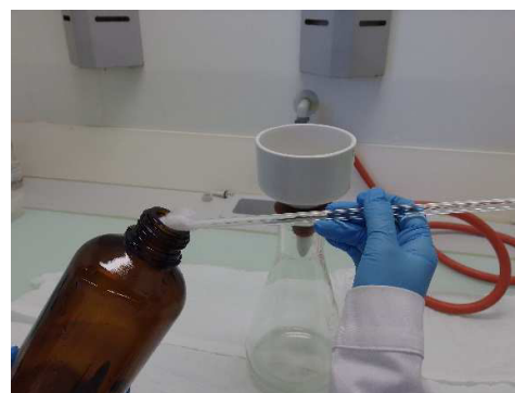
Fig. 3: Wiping the sample container with cotton wool soaked in solvent.
