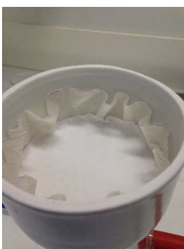
Fig. 2: Buchner funnel, muslin cloth and filter after passing Celite Hyflo Supercel solution through.
