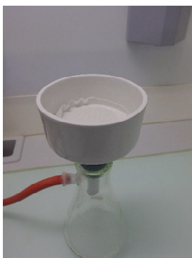
Fig. 1: Filtration flask with Buchner funnel, muslin cloth and filter.
