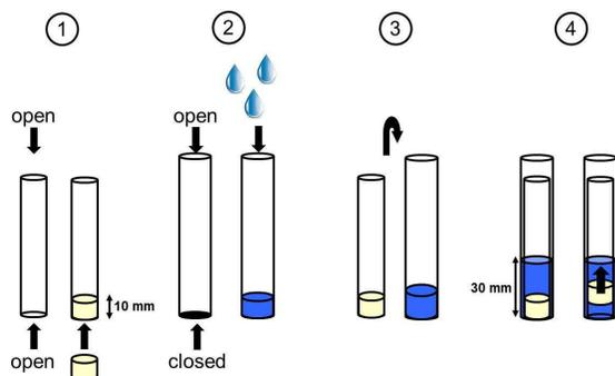
**Figure 1.** Illustration of the palm stearin sample preparation (steps 1-3) and the rising sample (step 4).
