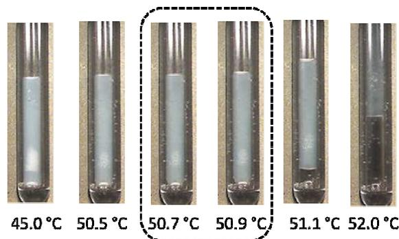
**Figure 2.** Snapshots of the palm stearin sample during the melting process. The SMP determined for six samples was  $50.7 \pm 0.1$  °C.
