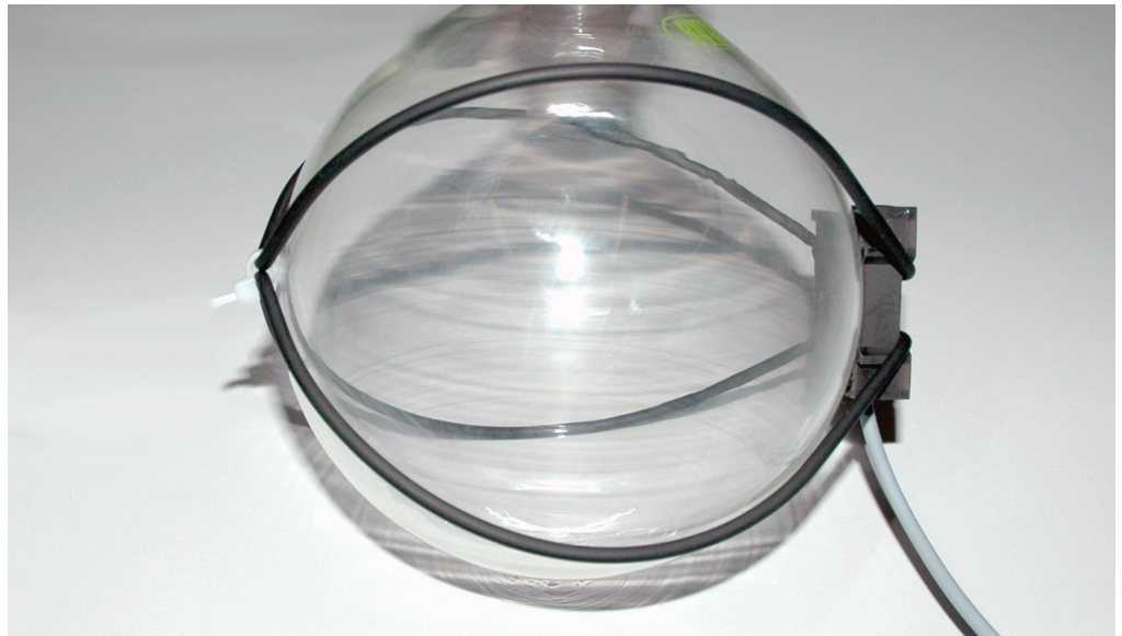
Picture 2: Attaching the level sensor to the flask
