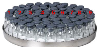
Figure 2: Steel shelf with the freeze dried mannitol samples.
