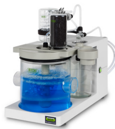
Scrubber K-415 Netralisasi
