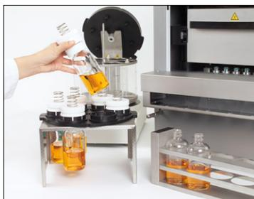
Sample transfer from SpeedExtractor to Multivapor™
