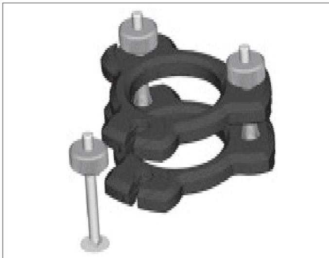
Figura 4.4: Montaggio EasyClamp
