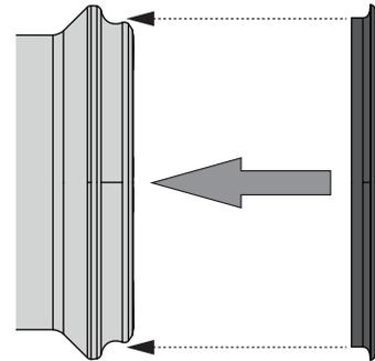
**NOTICE!** Depending on the instrument variation the seal can be different. The FatExtractor E-500 extended resistance comes with PTFE seals.
