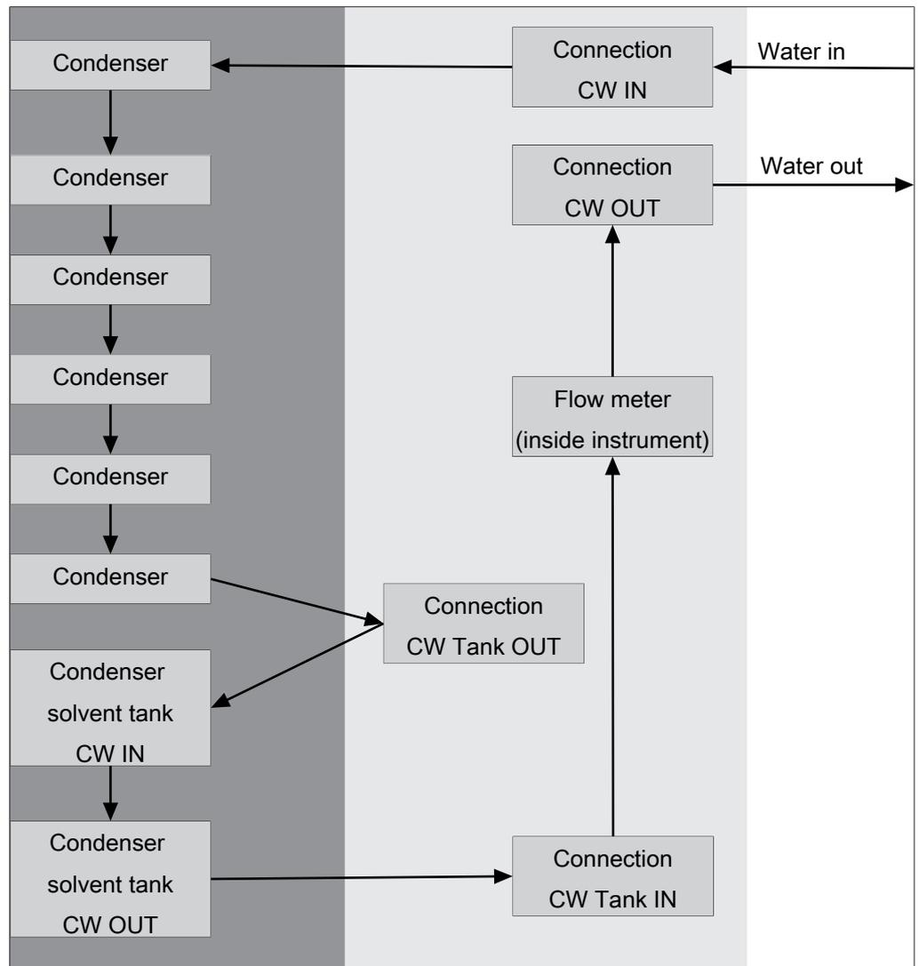
Fig. 16: Condenser circuit
