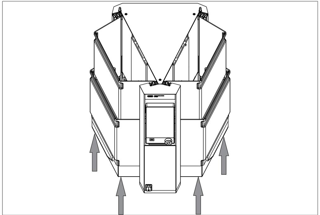
Fig. 10: Lifting the instrument
