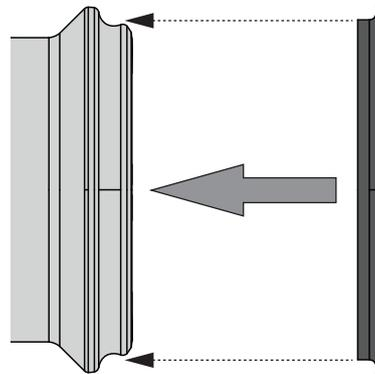
**NOTICE!** Depending on the instrument variation the seal can be different. The FatExtractor E-500 extended resistance comes with PTFE seals.
