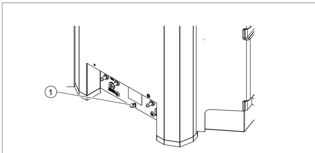
Fig. 11: Securing against earthquakes
