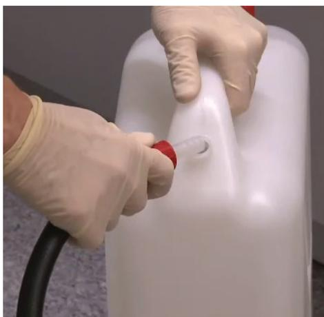
Bild 5.7: Connection of the drain hose using the straight connector
