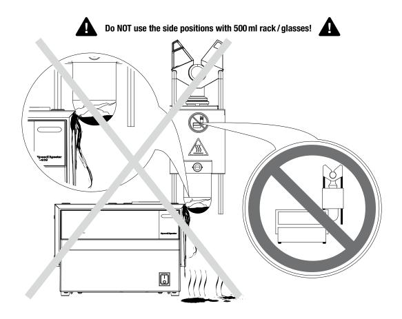
500 ml racks must be placed beside the SpeedDigester K-436 to avoid a crash between the sample tubes and the housing. Nonobservance will lead to hazardous situations especially when the sample tubes are filled and hot!
