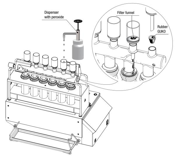
The funnels are placed decentralized (shifted out of the middle) above the sample tubes to prevent peroxide dripping directly into the hot sample. The filter funnel ensures that the peroxide can not flush into the hot sample to avoid dangerous deflagration of the peroxide and the sample.
