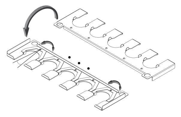
The 500 ml tube rack is equipped with a tube holder containing five sample tube support springs. Each flat spring must be freely rotatable by a small amount. If swivelling is not possible, exchange the rake!
