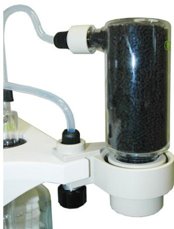
Fig. 5.16: Adsorption vessel with activated charcoal and glass wool
