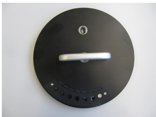
Fig. 3.3: USP standard plate for measuring cell NIRFlex Solid Transmittance cell
