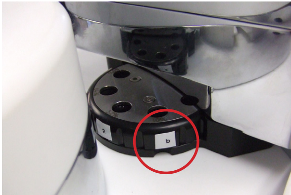
Fig. 6.17: Measuring position marked on the standards disk, an example of BREOS measuring position
