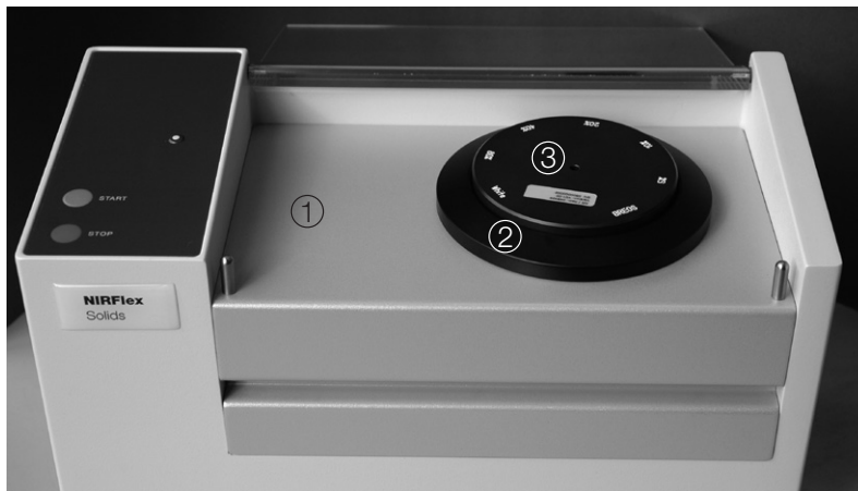
① Measuring cell NIRFlex Solids ② Standards add-on
