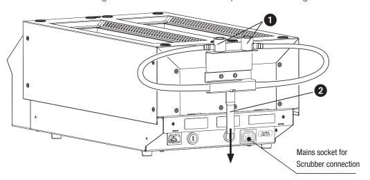
To connect a Scrubber/water jet pump the plastic adapter piece must be installed to the suction module and the hose connector must be mounted at the EPDM hose of the suction module (1) (see section 6.7.3).
