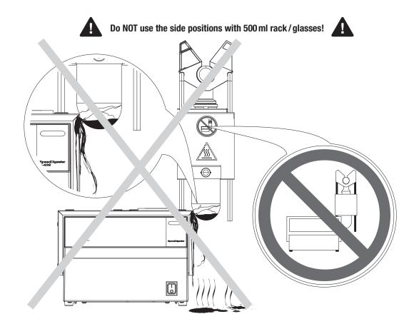
500 ml racks must be placed beside the SpeedDigester K-439 to avoid a crash between the sample tubes and the housing. Nonobservance will lead to hazardous situations especially when the sample tubes are filled and hot!
