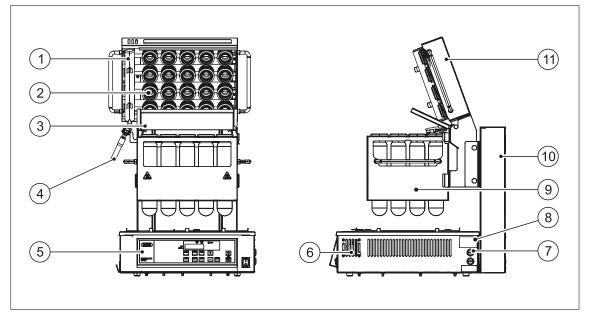
Fig. 4.1 KjelDigester front and side view
