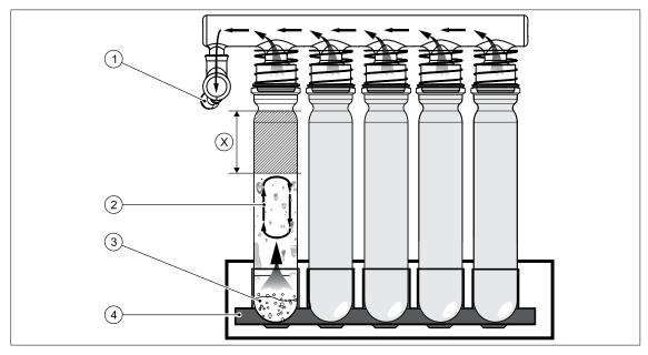
Fig. 4.4 Function of the KjelDigester
