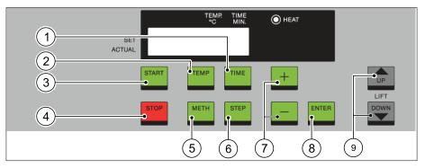
Fig. 4.6 KjelDigester K-449 control panel
