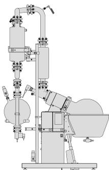
The “Continuous” setup contains a shorter but equally efficient condenser and one receiving flask. It is based on the descending configuration.
