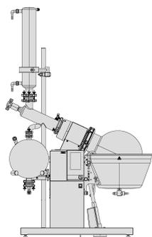
The “Essential” version is equipped with a vertical condenser and one receiving flask with a volume of 10 L. This configuration covers all the basic distillation needs. It is not recommended for bumping or foaming samples and also distillations under reflux are not possible.
