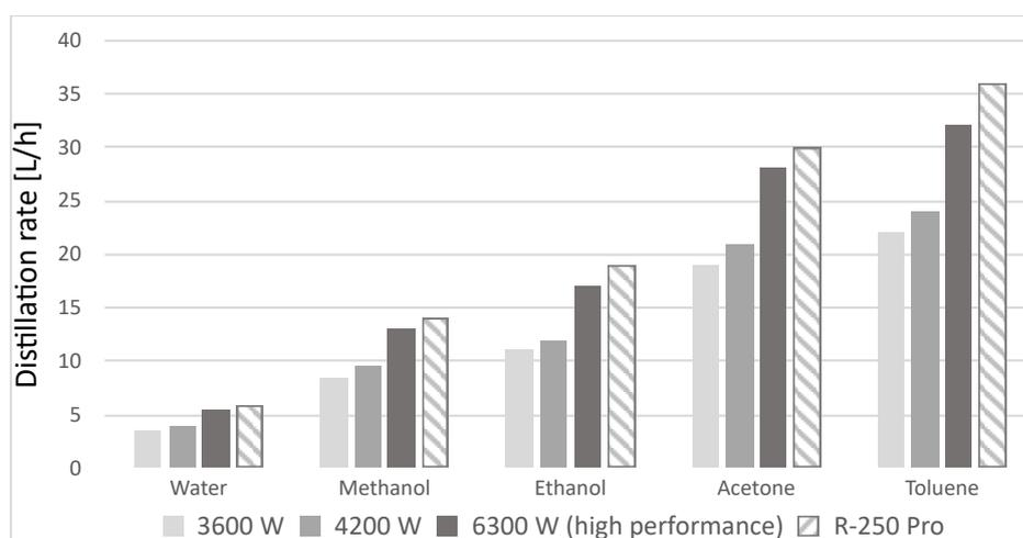
The maximum achievable distillation rate is not just related to the heating capacity, but also on rotation speed, flask size and temperature difference between bath and cooling.
