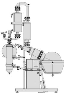
The R-220 Pro Extraction is based on the Standard R-220 Pro with a descending condenser, 1 receiving flask and the special 4 liter extraction chamber. It is designed for continuous cold extraction of natural products.
