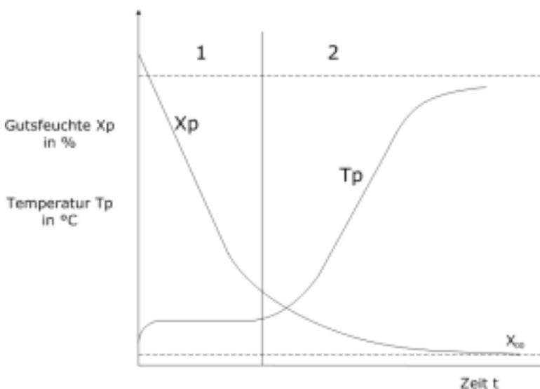
The diagram above shows that moisture content decreases significantly over time,  $t$ , until it reaches an equilibrium value. The temperature of substance  $T_p$  increases until it reaches the value of
