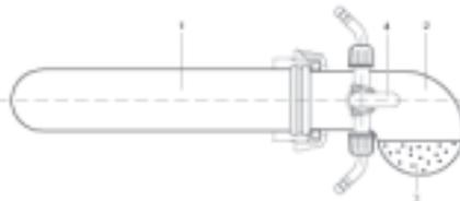
The drying oven is then operated in vertical position. The advantages of this method is that it avoids the need to transfer the sample into another container and that the sample container may be closed immediately.
