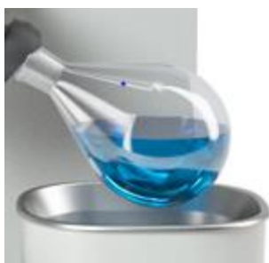
Figure 2: Optimum filling quantity is 1/3 to 1/2 of the evaporating flask' volume.
