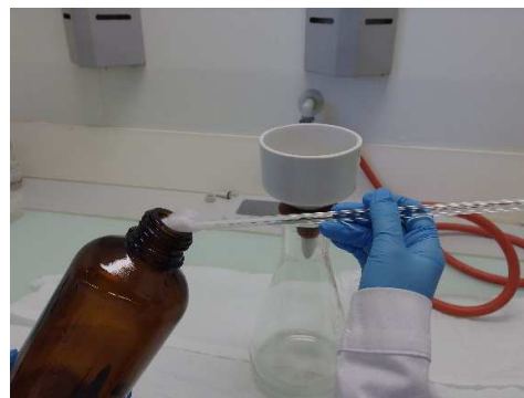
Fig. 3: Wiping the sample container with cottonwool soaked in solvent.
