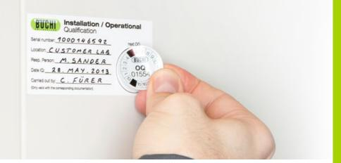
The Installation Qualification «IQ» provides the documented proof that the equipment has been delivered and installed in accordance with the requirements and statutory safety regulations stipulated in the design qualification. After a successfully completed Installation Qualification «IQ», the responsible persons release the equipment for the next stage of qualification. Typically an Operational Qualification «OQ».
