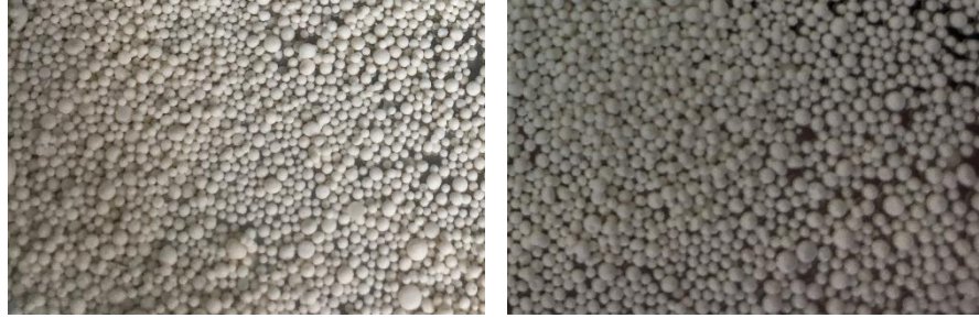
Figure 2: Yeast microbeads produced with the Encapsulator B-390 and the 300 \mu\text{m} nozzle before (left) and after (right) freeze drying
