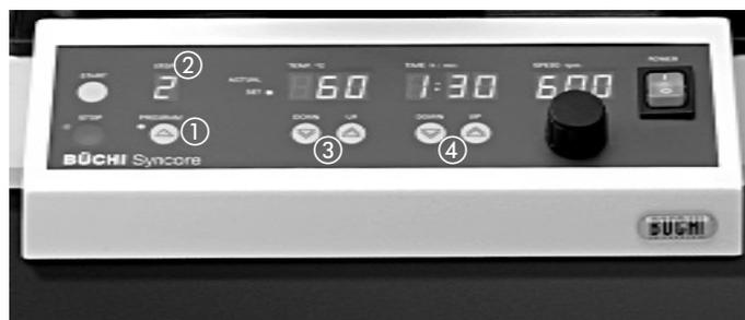
Figure 14: Display of the basic unit after starting up the equipment
