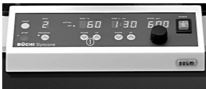
Figure 15: Display of the set-point temperature for the vacuum connection
