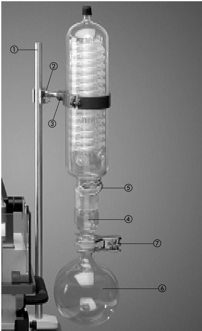
Figure 10: Attachment of the condenser unit
