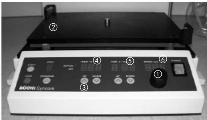
Figure 9: Controlling the basic functions from the control panel
