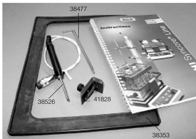
Figure 31: Replacement parts for the single platform
