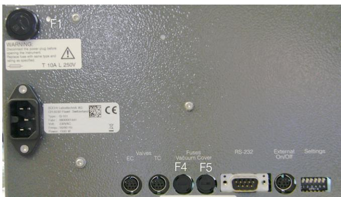
Figure 17: Signal-outputs and fuses with the corresponding order number qty 10) for the new Syncore setup.
