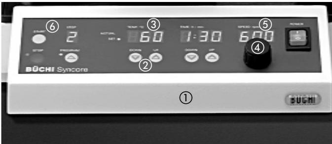
Figure 13: Display of the basic unit after starting up the equipment
