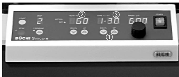
Figure 19: Display of the post-program running time
