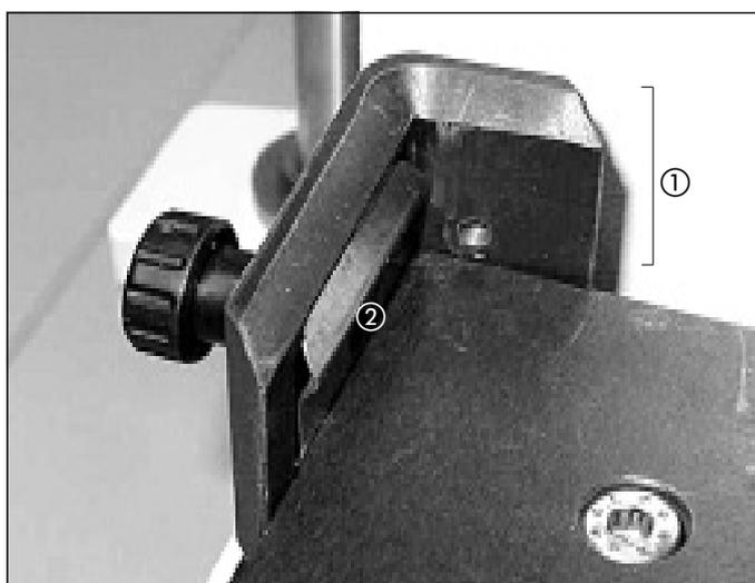
Figure 26: Corner brackets and springs
