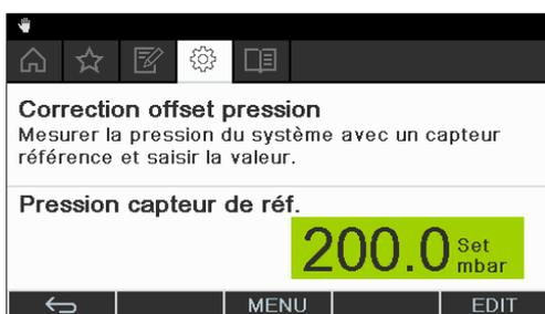
Fig. 57: Point de menu "Correction offset pression"
