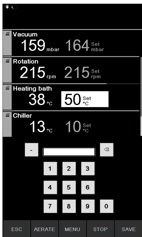
Fig. 30: Editing parameters while distillation is in progress
