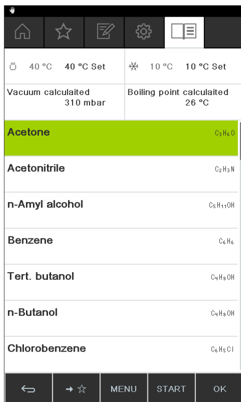
Fig. 57: Selecting "Set" temperature for heating bath when using equipment of a different make
