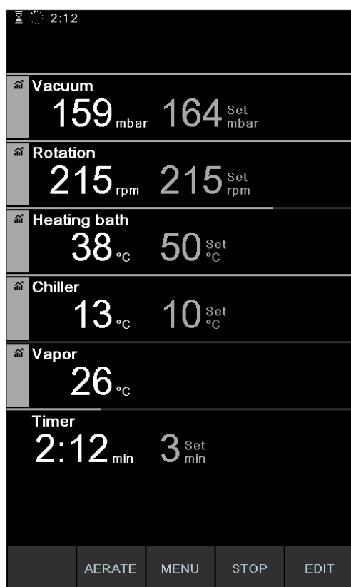
Fig. 33: "Timer" screen while distillation is in progress
