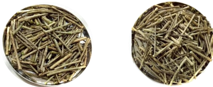
Figure 1 : Giloy stem before (left) and after (right) freeze-drying
