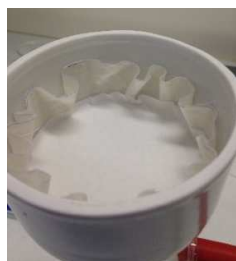
Figure 2: Filtration flask with Buchner funnel, muslin cloth and filter.
