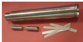
Fig 1: 10 mL extraction cell, two expansion elements and the sample, cut in strips [6]
