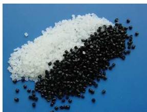
Figure 1: Polyamide PA 6 (black), Polyamide PA 12 (white).
