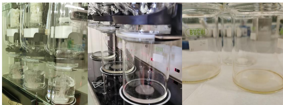
Figure 1-5: Pulp sample during extraction (left), after drying (middle) in E-800 and after drying in drying oven (right)
