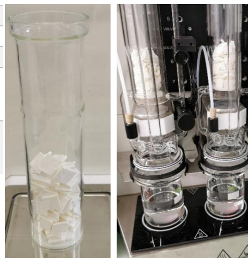
Figure 1-2: Sample tube filled with sample (left) and placed into the extraction chamber (right)
