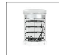
Acrylic chamber with heated shelves for bulk and vial drying.
