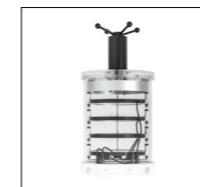
Acrylic chamber with heated shelves and stoppering for vial drying.
