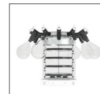
Acrylic chamber with 12 manifold top and shelves for bulk, vial and flask drying.
