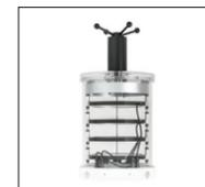
Acrylic chamber with heated shelves and stoppering for vial drying.
