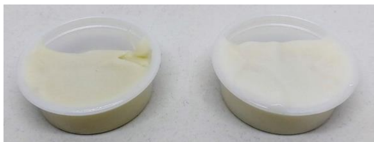
Figure 7. Result of an optimized activated carbon decolourisation on an extract of Quercus pubescens without decolourisation (left) and decolourised (right) formulated at 3%
