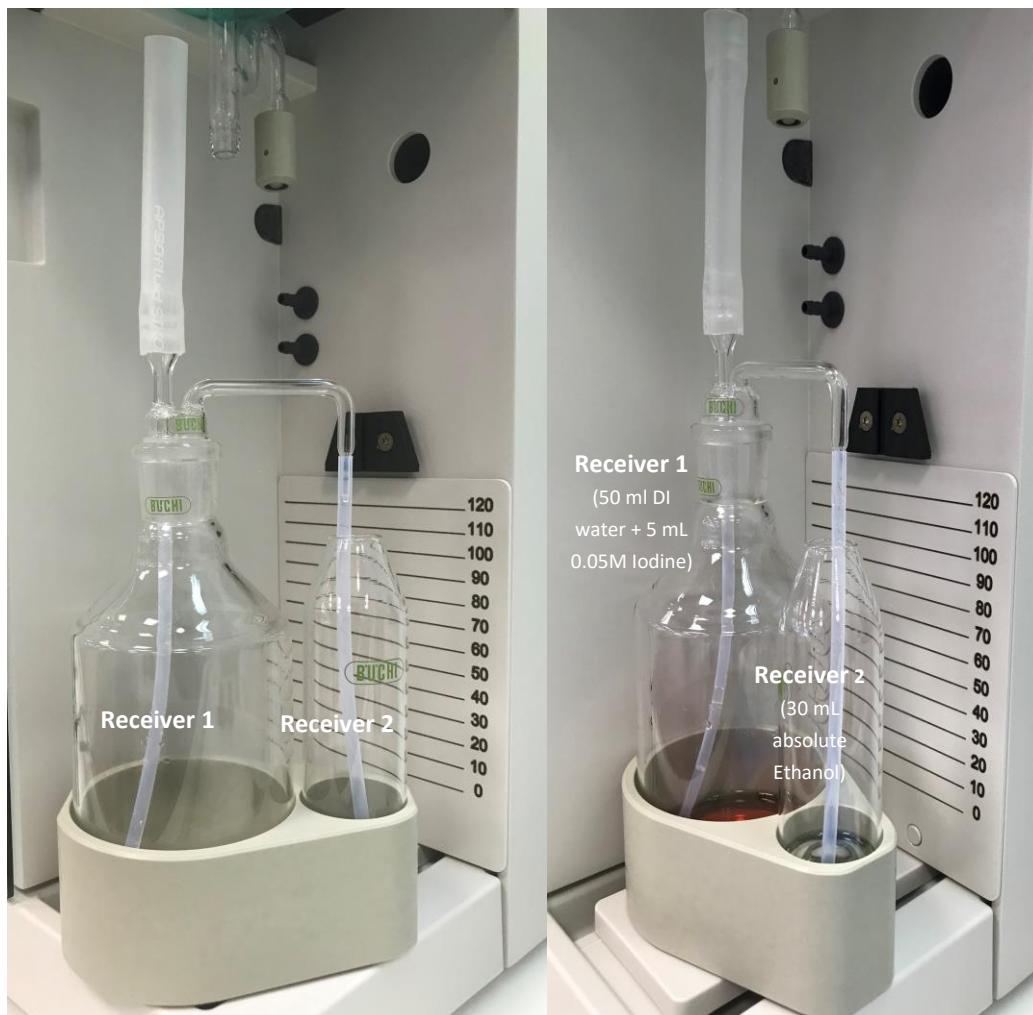
Figure 1: BUCHI SO 2 absorption glass set (left), BUCHI SO 2 absorption glass set with relevant solutions in Receiver1 and Receiver2 correctly attached to the distillate outlet (right)
