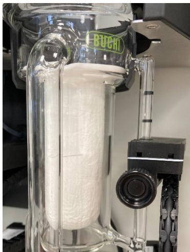
Figure 5: placing the level sensor according to the pencil mark at filter paper's height.
