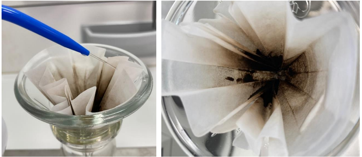
Figure 3 (left): Rinsing of the filter paper. Figure 4 (right): sample in the filter after the hydrolysis.
