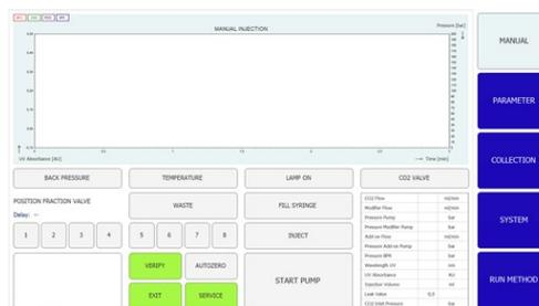
▶ Tap the *[Verify]* button to ensure that all modules are communicating correctly.
