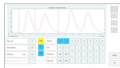
**NOTICE! The method for the fractionation (time and/or peak based) as well as the Start peak detect time can not be changed after the run is started. These buttons are just for information.**
