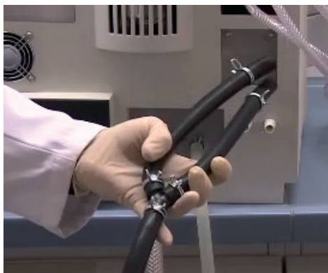
Fig. 5.6: Guidance of the two outlets into one hose
