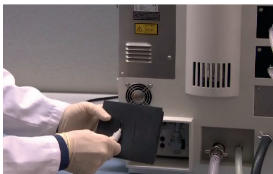
Fig. 5.10: Guidance of the cable through the cut-out
