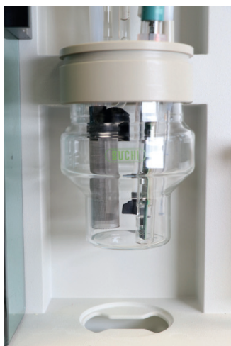
Fig. 5.17: Colorimetric titration setup
