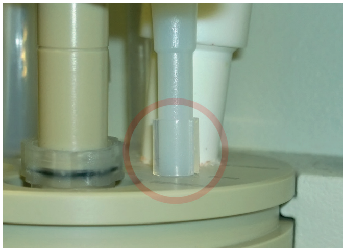
Fig. 5.12: Mounting of the spacer at the dosing tip
