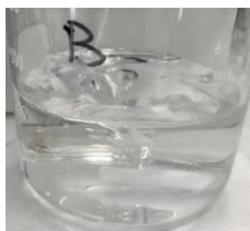
Figure 3: Distillate before titration with 0.02 N ammonium thiocyanate standard volumetric solution (transparent).
