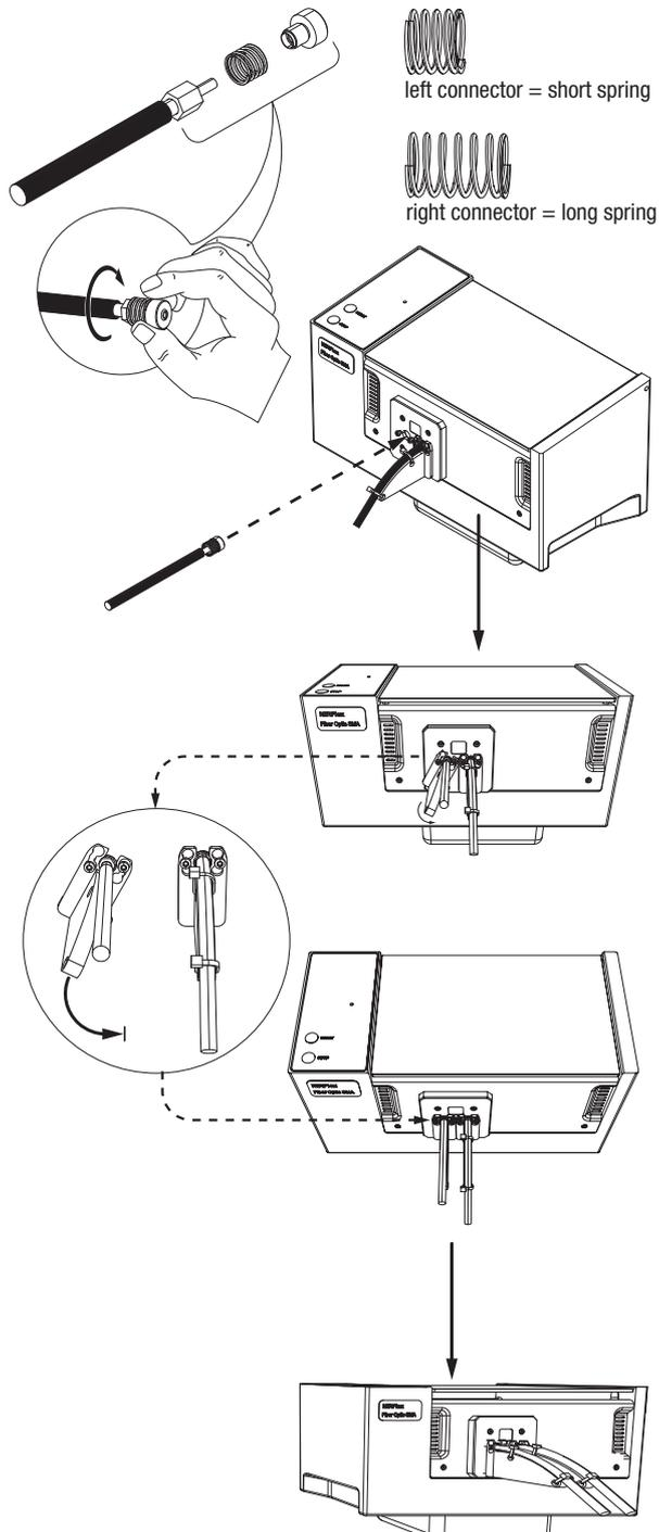
To mount the SMA-adapter onto the optical fiber cable:
