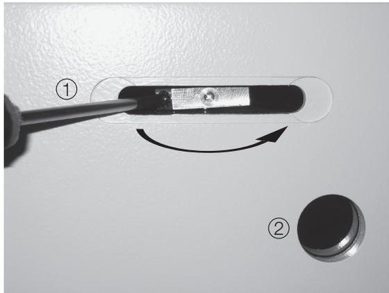
In the front of the main cover of NIRFlex N-500 there is an opening which is hidden behind the "Locked - Unlocked" shield. For the operation of the transportation lock pull out the shield first. Insert the torx screwdriver supplied with the instrument and flip the locking mechanism by moving it to the side.
