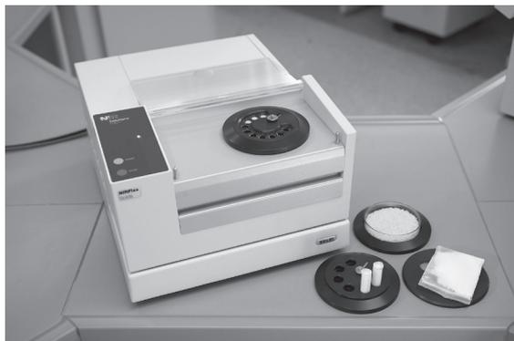
The NIRFlex Solids is the ideal configuration to measure solid samples like powders, pastes and pellets in diffuse reflection mode. The measuring cell for solids allows the use of different add-ons for specific sample containers.
