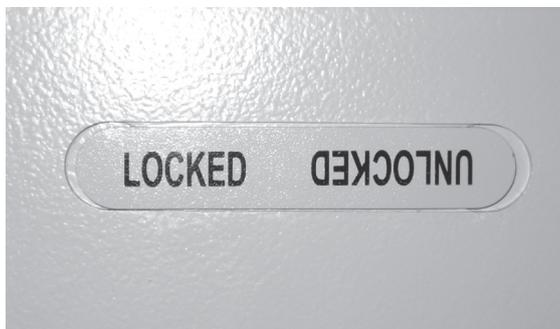
The installation position of the shield depends on the locking status of the transportation lock. The label of the shield in this image indicates a locked transportation lock.
