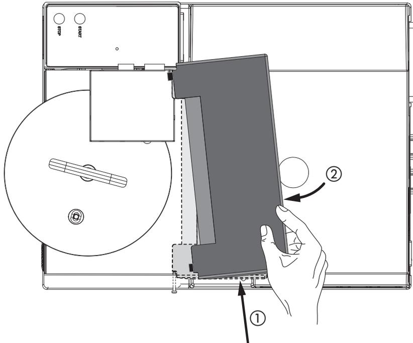
Insert the tilted cover ① and hook its left hinge onto to the bushing pin (hinge counterpart) at the rear left hand side of the measuring cell. Tilt the cover back into a straight position ②.
