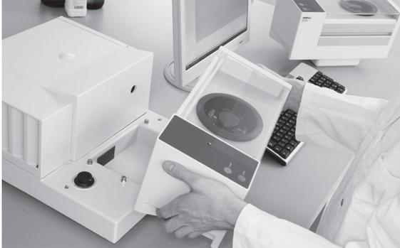
Installing a measuring cell
