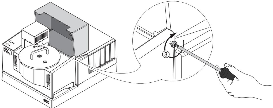
Keep the right hinge of the cover in a matching position with the bushing screw. Fasten the screw ③ with a few turns (the screwdriver is part of the scope of delivery). Open and close the cover several times to verify the correct installation.
