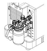
▶ Attach the vacuum hose to the condenser.
