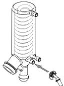
▶ Attach the hose to the secondary condenser.
