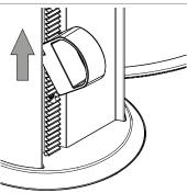
▶ Lock the position of the height adjustment stopper.
