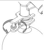
▶ Remove the ball joint clamp.
