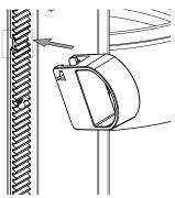
▶ Move the rotary drive arm to the desired lowest lift height.
