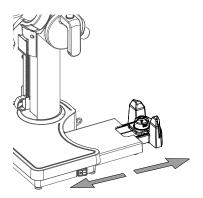
▶ Position the heating bath on the instrument base.
