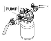
► Attach the hose to the vacuum pump connection IN.
