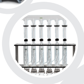
Water reflux setup
