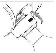
▶ Remove the evaporating flask from the vapor duct.
