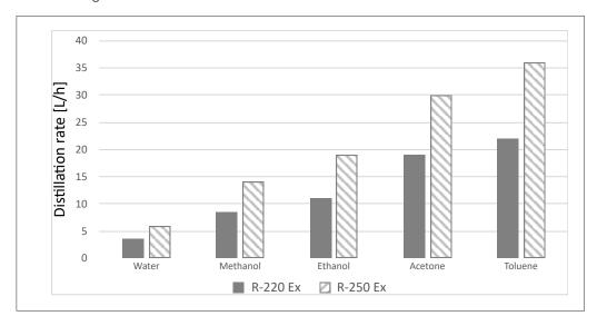
The maximum achievable distillation rate is not just related to the heating capacity, but also on rotation speed, flask size and temperature difference between bath and cooling.
