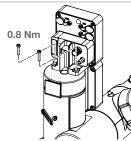
► Re-install the mounting fixture.
