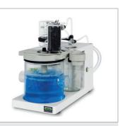
The Scrubber K-415 with up to four cleaning steps provides maximum safety for operator and environment.
