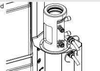
Make sure that the solvent collector circuit is complete. See Chapter 11.1 "Schematics", page 75
