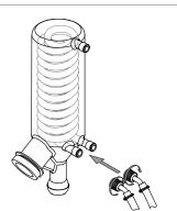
► Attach the coolant hoses to the Chiller/Cooling.
