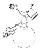
▶ Turn the wheel to secure the ball joint clamp.
