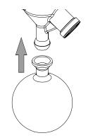
Secure the receiving flask with the ball joint clamp.
