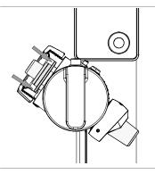
▶ Insert the condenser into the flange nut.
