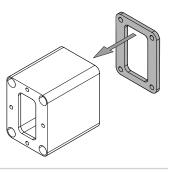
Pass the USB-C cable and the power cable through the cable seal fixture.
