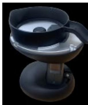
Place sample cup on top of rotator.
