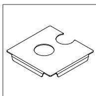
Fig. 6: Positioning plate with two openings for up and down view
