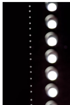
Generation of a stable, vertical droplet chain.
