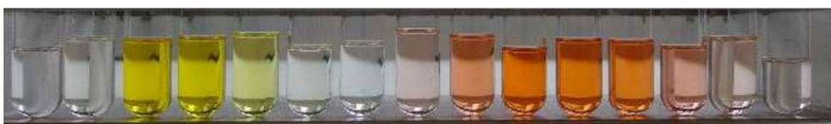
Figure 2: Separated and collected dyes. a): separation with gravity column chromatography. b): separation by flash chromatography using Pure Essential.
